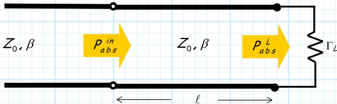
Recall, however, that a lossless transmission line can absorb **no** power! By adding a length of transmission line to load  $\Gamma_L$ , we have added only **reactance**. Therefore, the power absorbed by load  $\Gamma_{in}$  is **equal** to the power absorbed by  $\Gamma_L$ :
